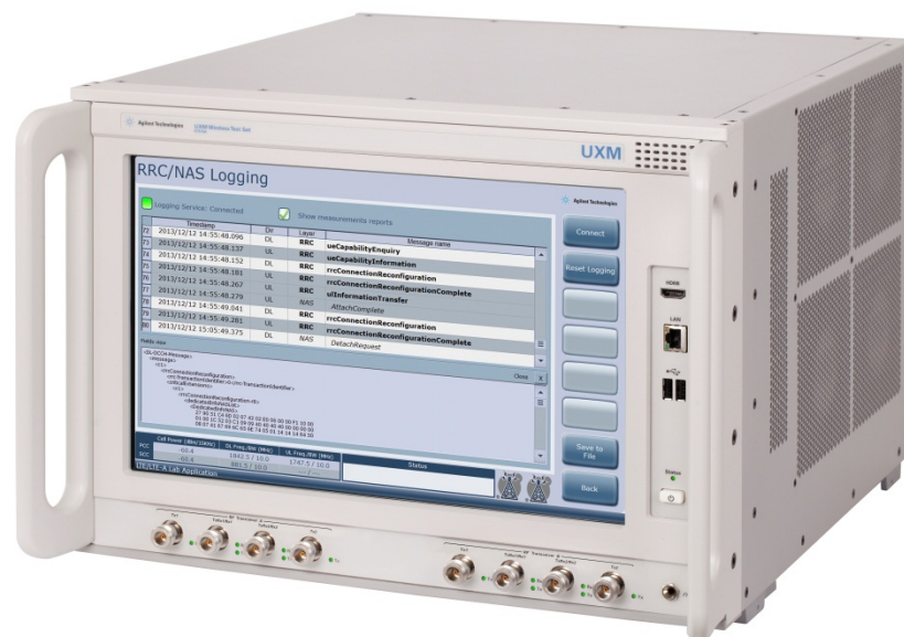
Figure 1-1 Agilent E7515A UXM Wireless Test Set
